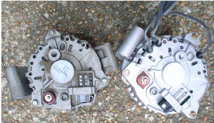
*The alternator on the far left is the OEM unit, while the one next to it and on the far right is the upgraded HD unit from Quick Start. You can see the pre-installed wiring which connects the new alternator's internal rectifier to the additional fan-cooled remote Rectifier box (Quicktifier).*
