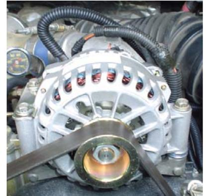
Installation wasn't bad, but the kit did not include the necessary 4 AWG cables for running from the new alternator to the rectifier box and then to the battery. Also, there was no wiring diagram for those without a solid grasp on all the electrical implications of this upgrade, so I included a simplified version of mine below for reference. Other unexpected issues I faced were:
