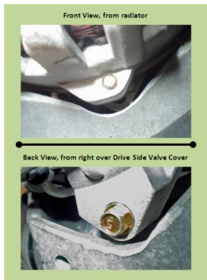
Minor Bracket Grinding or Shims under the mounting feet.
