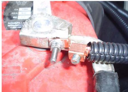
200 amp ANL fuse block between Quicktifier and Battery (driver side).
